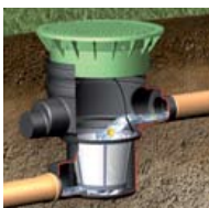
Sedimentation filter shaft fitted flush with the ground, with outflow to infiltration tunnel
