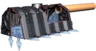
Cut-away section of percolation tunnel showing the inflow and percolation of stormwater
