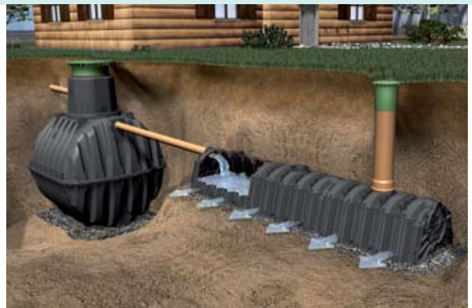
Percolation tunnels shown as a soakaway.
